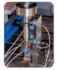
Note: Two of the sensors (Y Y2) are located behind the dualmasterball target.
