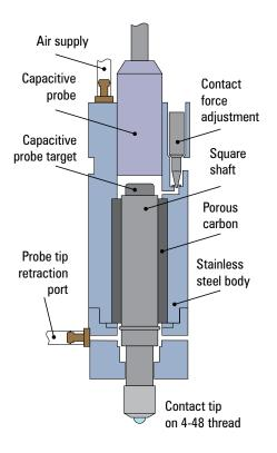
The calculations here are based on a 6.9 g moving mass of a C-LVDT (5.55 g Shaft, 1.35 g Tip). Shorter, older models (no longer available) had lower mass and slightly higher response speeds.
